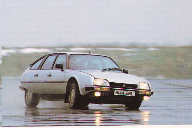
CITROEN'S CLASSIC SHAPE HASN'T DATED MUCH IN A DECADE, BUT CABIN IS OUTDATED AND WILL SOON BE REVISED. TURBO ENGINE HASN'T QUITE THE STUFF OF ROVER OR BMW, BUT CX IS STILL A FAST CAR. HANDLING IS FAIL-SAFE FWD, WITH UNDERSTEER AT LIMIT. STABILITY IS EXCELLENT
