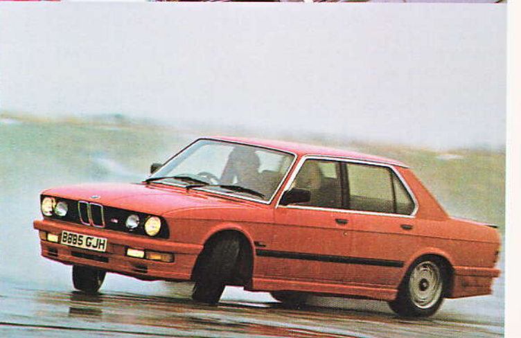
MATRONLY LINES OF M351 BELIE SPORTY CHARACTER OF CAR. CABIN APPOINTMENTS ARE THOSE OF LUXURY FIVE SERIES, WITH SMALL WHEEL AND SPORTS SEATS THROWN IN. ENGINE IS 218BHP UNIT FROM 735I AND 635CSI. IT'S SMOOTH, PUNCHY, FLEXIBLE. OVERSTEER IS EASILY CONTROLLED
