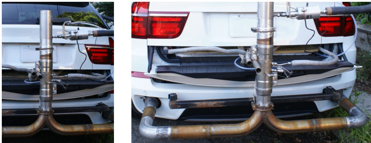
Figure 3.26: Exhaust adapter setup for Vehicle C, left: 3.5" exhaust flow meter (EFM), right: joining double vehicle exhaust stack into exhaust transfer pipe
