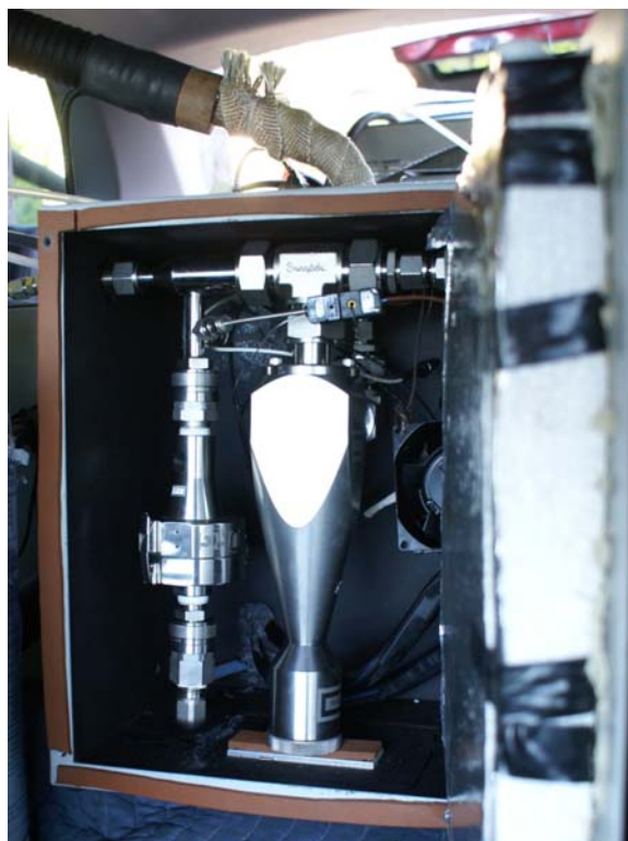
Figure 3.27: Horiba OBS-TRPM heated filter holder box for gravimetric PM quantification, sample is introduced from the top, left: 47mm filter holder, right: 2.5 cut-point cyclone
