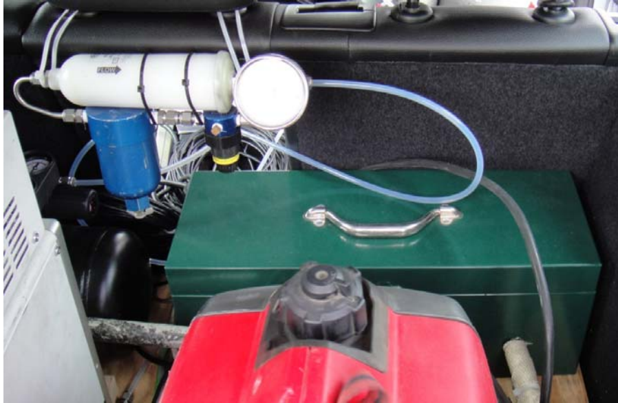
Figure 3.30: PPS setup, the sensor is housed within the green box, top left: pressurized, dried and HEPA filtered air supply for PPS
