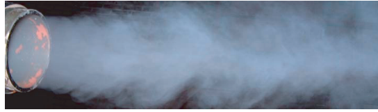
Figure 6.4: Smoke visualization of jet mixing layer at Reynolds number of 65,000.
