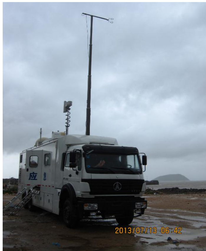
Fig.2.5 2 nd generation typhoon observing vehicle developed by Shanghai Typhoon Institute
