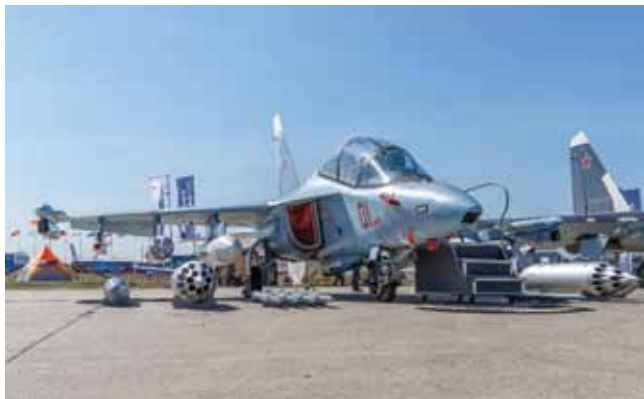
Modified Yak-130 in strike configuration with laser rangefinder clearly visible on the nose, on static display at MAKS-2015
