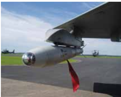
A clear view of the infrared seeker on an MBDA ASRAAM missile
