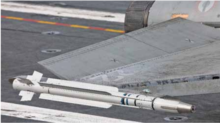
An IR variant of the MBDA MICA mounted to the wingtip station of a French Navy Rafale M
