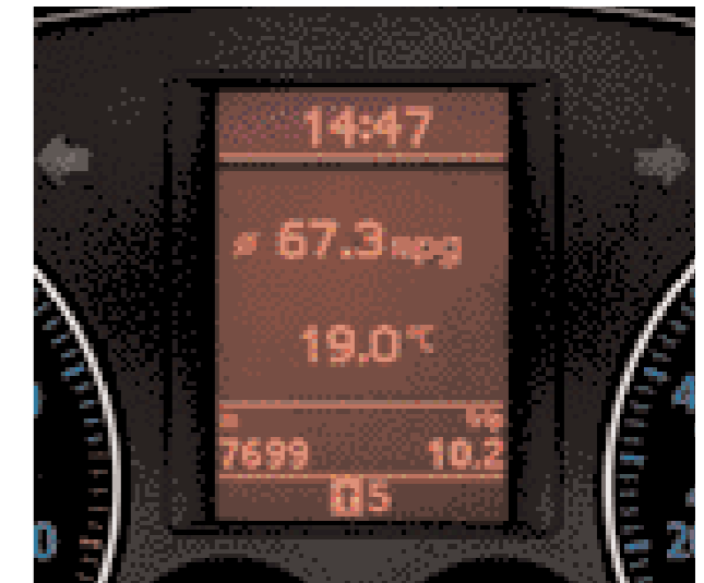
The multifunction computer (Highline) includes visual gear change recommendation for optimum fuel consumption. Standard on BlueMotion Passat models.
