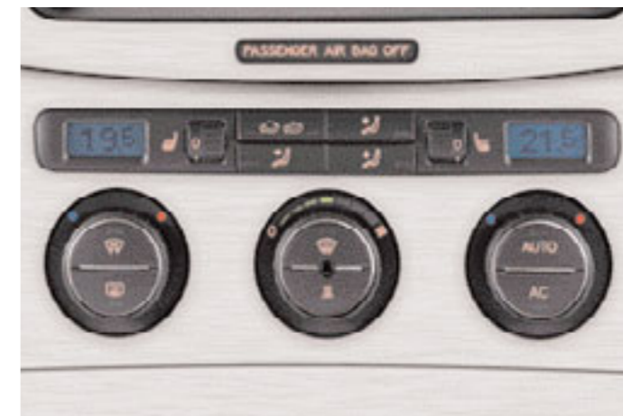
2Zone electronic climate control with an automatic air recirculation feature produces a pleasant, consistent temperature.
