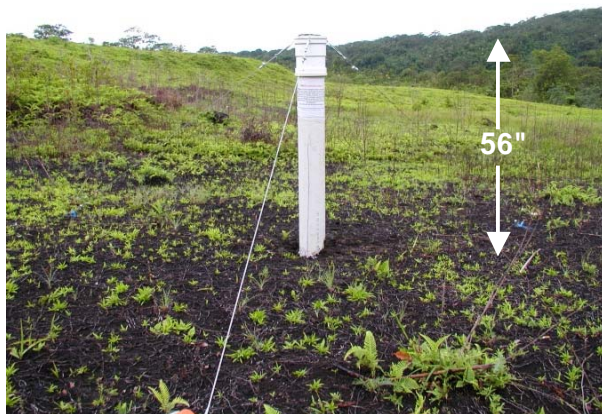
Figure 5. (a) A view of the specially designed 56-inch PVC pipe rain gage assembled in the field at the Mahnd site on Pohnpei Island. (b) A view of the recording tipping bucket rain gage assembled in the field at the Nihpit site on Pohnpei Island.
