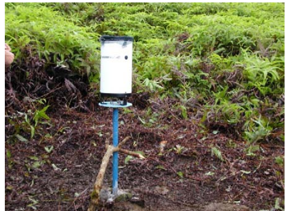
Figure 5. (a) A view of the specially designed 56-inch PVC pipe rain gage assembled in the field at the Mahnd site on Pohnpei Island. (b) A view of the recording tipping bucket rain gage assembled in the field at the Nihpit site on Pohnpei Island.
