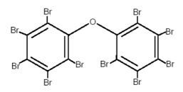
A typical composition for a modern flame retardant product would be 97-98% deca-BDE with 0.3-3.0% of other brominated diphenyl ethers, mainly nonabromodiphenyl ether, and the composition of products supplied in the EU is consistent with these figures.
