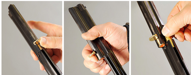
Reloading a Henry repeater: (1) Follower tab full-forward and locked, (2) barrel tip twists open, (3) rounds inserted into magazine
