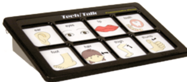
Figure 12. 3. Example of a speech generating devise.
