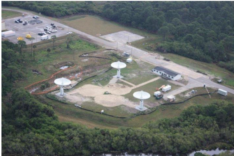
Fig. 1. Overhead shot of the KaBOOM site at the Kennedy Space Center. It is comprised of three 12m diameter antennas. The operations center is seen just to the right of center. Spacing between the antennas is 60m.
