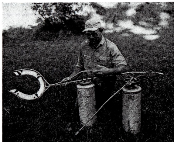
Figure 1. Equipment for basal spraying red alder.
