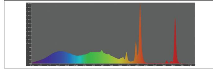
Figure 2. SPD of a typical CRT.
