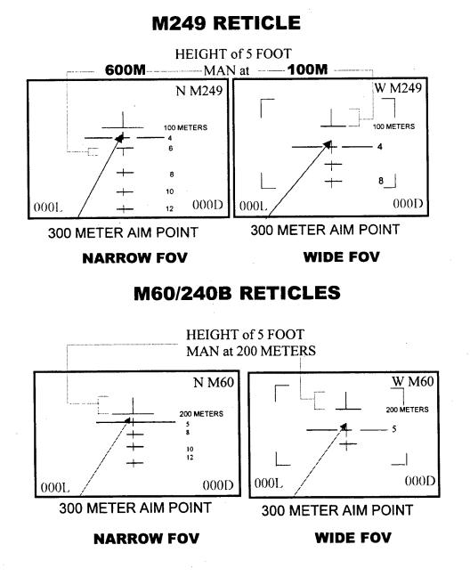
*Figure 18.* TWS reticles for the M249 and M240B. [Not to scale. The labels "100 meters" and "200 meters" were included on the viewgraphs for instructional purposes. They are not in the TWS reticle.]
