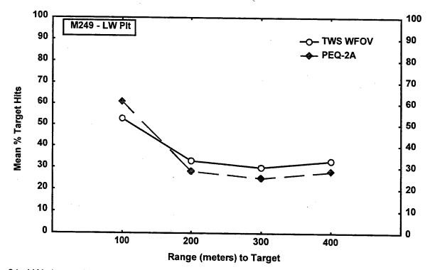
Figure 21. LW platoon M249 qualification by range to the target.
