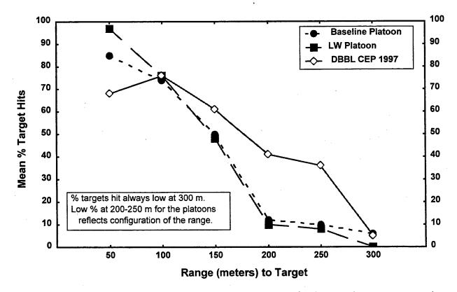
*Figure 17.* Percentage of target hits by range with aiming lights for the two platoons compared to a prior test by the Dismounted Battlespace Battle Lab.
