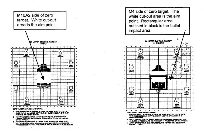
*Figure 5.* M16A2 and M4 sides of the 25-meter zero target configuration for the TWS on the M4 carbine.
