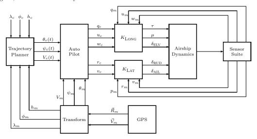
Figure 7. Control System Block Diagram
