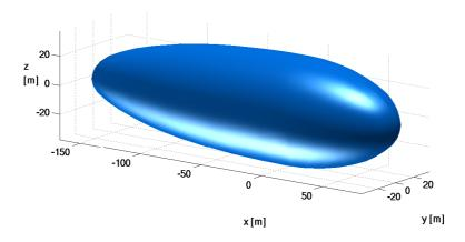
Figure 2. 3D View of Double-Ellipsoid Hull Geometry
