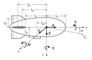
Figure 5. Steady-State Aerodynamic Model
