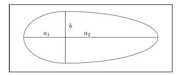
Figure 1. Double-Ellipsoid Geometry for Airship Hull
