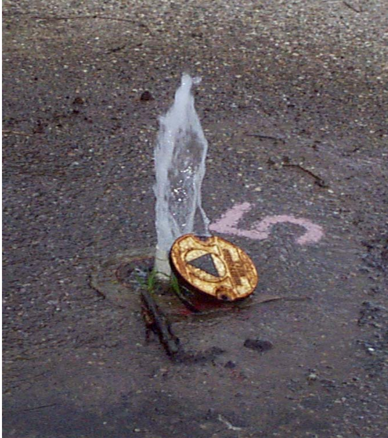
Figure 14. Geysering Effect Following an Increase in Air Injection Rate
