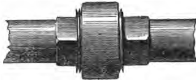
GENERAL VIEW OF COUPLING AND UNION.
