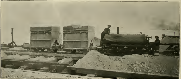
STEAM ORE CARS. Used in connection with steel gallows frame.
