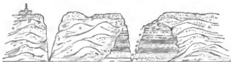
a. Shale and sands. b. Black shale, with calcareous concretions and fossils. c. Thickly laminated sandy marl and greensand. d. Dark shale. e. Yellowish ferruginous sands, with concretions of calcareous grit or sandstone loaded with Ammonites, Belemnites, and other fossils. f. Dark-coloured marls, followed by others of yellowish tint and sandy and ferruginous structure, with courses of marlstone, &c. These regular beds are covered by argillaceous drift (g), which for the most part obscures the section.
