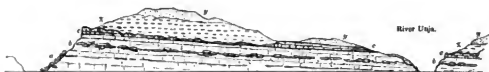
a. Limestone, concretionary. b. Yellowish and magnesian limestone, with thinly laminated bands of fit and ochreous argillaceous way-boards. The rock is very cavernous, and the cavities are often lined with corals, chiefly a large Cyathophylidium ; and among the other fossils are Orthis eximia , Productus comoides , P. undatus De Fr., P. antiquatus , Spirifer Mosquensis , Leptaena Hardensis , with Echini . These beds are covered on the surface, and their superficial depressions filled with iron sand are succeeded at a little distance in the cliff by a white, hard, flag-like, sandy limestone (c). The iron sands (c), which cover indistinctly the denuded beds of limestone and the drift (g), will be described in subsequent chapters.
