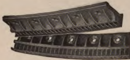
REVOLVING BUCKETS FOR CURTIS STEAM TURBINE.
