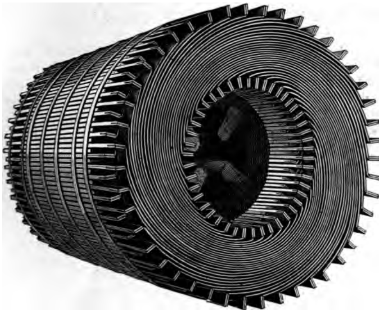
CROMPTON AND SWINBURNE'S DRUM-ARMATURE.
