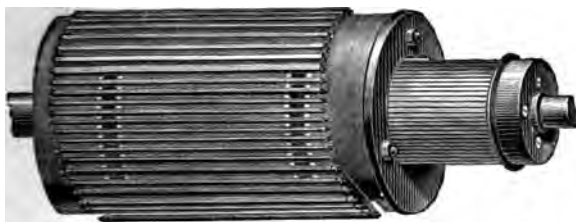
ARMATURE OF EDISON DYNAMO.
