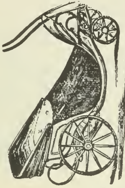
No. 17 is a four-wheeled Victoria Pleasure Ground Chair, mounted in a very light iron framed carriage, upon c and patent India-rubber springs, is either drawn by hand or animal, and is the most elegant and easiest chair made.
