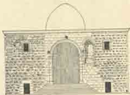
Fig. 143. Restoration of façade of kalybê at il-Haiyât.
