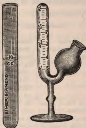
FIG. 1.—Einhorn's fermentation saccharometer. The fermentation saccharometer can be obtained at Eimer & Amend, 205 3rd. Ave., New York.
