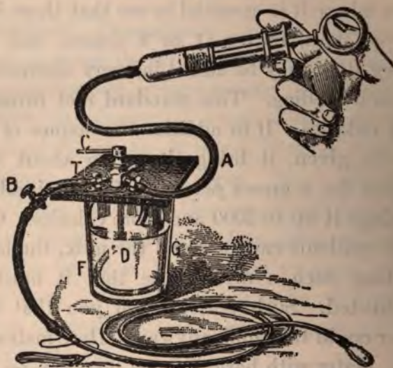
FIG. 6.—The duodenal feeding apparatus, with table support. A, tube leading to syringe; B, tube leading to duodenal pump; C, crank; D, tube leading to fluid; F, fluid; G, glass; T, table support or shorter support. When crank C is turned parallel to A, fluid can be aspirated from the glass into the syringe. When C is moved parallel to B, the fluid from the syringe can be emptied into the duodenum.
