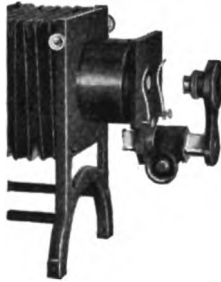
FIG. 173. BAUSCH & LOMB'S SIMPLEST FORM OF PROJECTION MICROSCOPE. (Cut loaned by the Bausch & Lomb Optical Co.).
