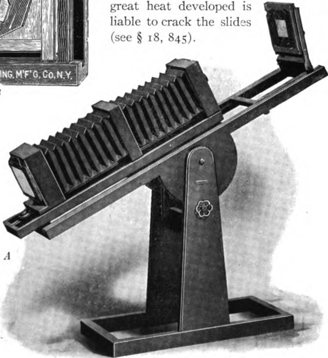
FIG. 119. FOLMER & SCHWING'S TILTING CAMERA AND ADJUSTABLE BACK.
