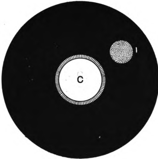
FIG. 195. SHIELD AT THE END OF THE ARC LAMP CONDENSER TUBE TO AID IN CENTERING THE LIGHT.
