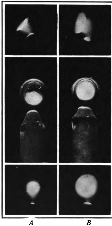
FIG. 294. FACE AND LATERAL VIEWS OF THE RIGHT-ANGLE CARBON ARC WITH 10 AND WITH 20 AMPERES OF DIRECT CURRENT.
