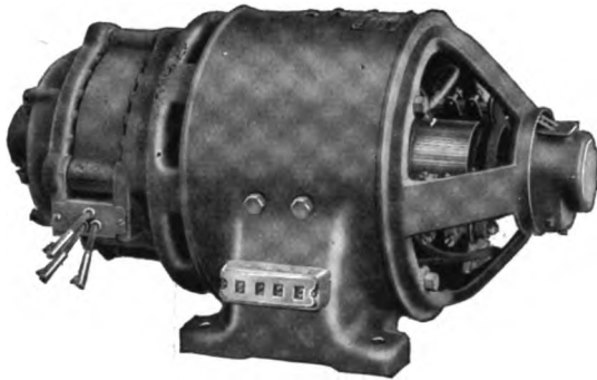
FIG. 258. MOTOR-GENERATOR SET. (Cut loaned by the General Electric Co.).
