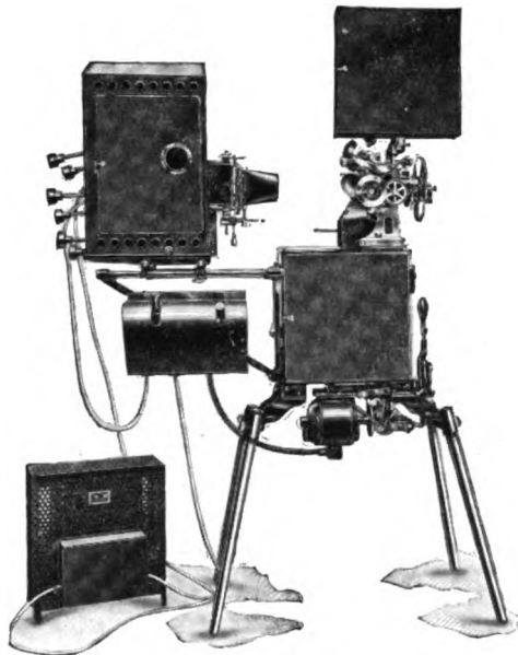
FIG 222.. POWER'S CAMERAGRAPH NO. 6, SHOWING THE LAMP-HOUSE IN POSITION
