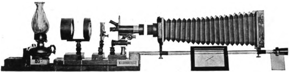
FIG. 219. MICRO-PROJECTION OUTFIT AND VERTICAL CAMERA ARRANGED FOR PHOTO-MICROGRAPHY.
