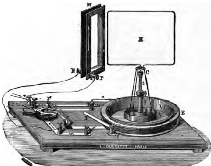
FIG. 71.—AMPERE'S FRAME, ARRANGED TO SHOW THE FORCES BETWEEN PARALLEL CURRENTS.
