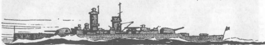
ADMIRAL SCHEER. "Pocket" battleship, 10,000 tons. Armament, six 11-in. guns, eight 5.9-in. guns, six 4.1-in. and eight 3-pdr. anti-aircraft guns. Speed, 26 knots. Carries a complement of 926. Completed November 12, 1934.
