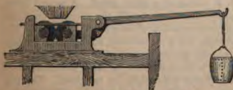
Fig. 135.—Showing mode of applying pressure on rollers.
