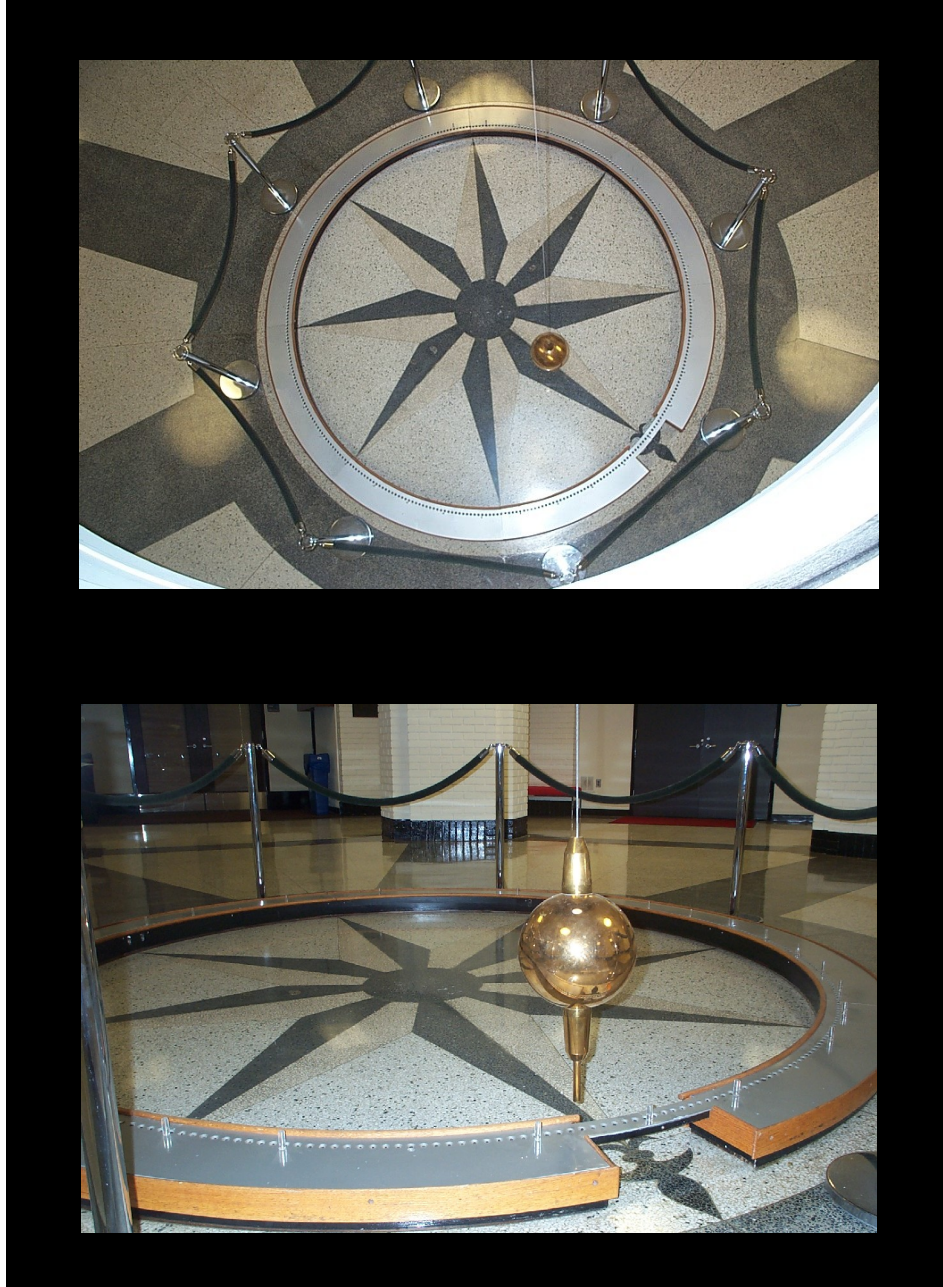
Figure 6: The Foucault pendulum in Grawemeyer Hall in Louisville, Kentucky (USA). Foucault's pendulum, introduced in 1851, was the first laboratory demonstration of the diurnal rotation of the Earth that could be widely and easily reproduced.
