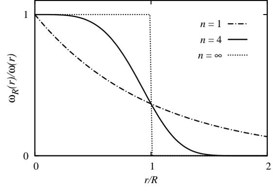
FIG. 1: Screening function  $w_R(r)/w(r)$  as function of the distance between the two charged particles  $r$  for characteristic values of the parameter  $n$  in Eq. (1):  $n = 1$  (dashed-dotted curve) corresponds to Yukawa screening,  $n = 4$  (solid curve) is the choice of this paper, and  $n \rightarrow \infty$  (dotted curve) corresponds to a sharp cutoff.
