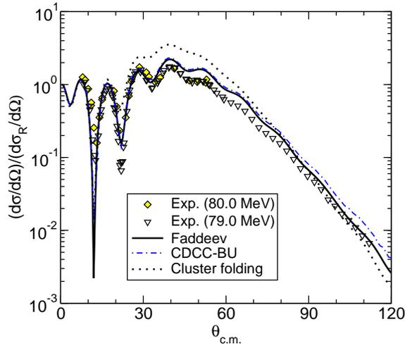
FIG. 6: (Color online) Elastic cross section for deuterons on  $^{58}\text{Ni}$  at  $E_d = 80$  MeV : the solid line corresponds to exact three-body results and the dash-dotted line to CDCC results. The experimental data at 80 MeV (diamonds) are from Ref. [23], and those at 79 MeV (triangles) are from Ref. [24]. The dotted line is the CDCC calculation suppressing the coupling to the deuteron continuum (see text).
