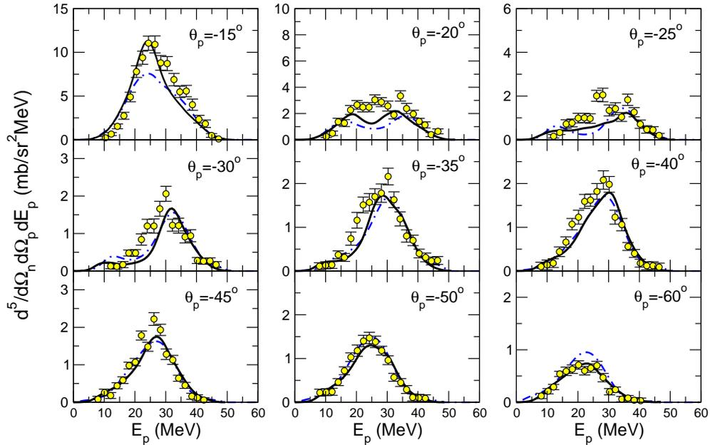
FIG. 5: (Color online) Exclusive differential cross section versus proton energy for the breakup of deuterons on  $^{12}\text{C}$  at  $E_d = 56$  MeV, for  $\theta_n = 15^\circ$  and  $\theta_p < 0$ : the solid line corresponds to exact three-body results and the dash-dotted line to CDCC. The experimental data are from Ref. [37].
