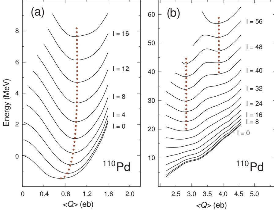
Fig. 1. Calculated energy surfaces in  $^{110}\text{Pd}$  for different angular momenta as a function of static quadrupole moment  $\langle Q \rangle$ . (a) Region I. The energy zero is set to be the total energy at  $\langle Q \rangle = \varepsilon_2 = 0$  and  $I = 0$ . (b) Region II. The absolute energy is arbitrarily chosen. Note that the plots do not give the relative energy between the two regions.
