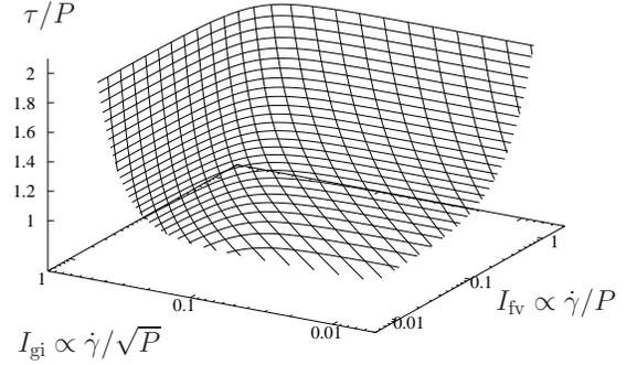
FIG. 3: Predicted response for a granular material in the crossover between the grain inertia regime and the fluid viscosity regime.  $\tau/P$  is the effective friction.  $I_{gi}$  and  $I_{fv}$  are given by Eq. (16). The “gi” and “fv” limits ( $\tau/P$  as a function of  $I_{gi}$  or as a function of  $I_{fv}$ ), represented on Fig. 2, are (approximately) given by the edges of the meshed surface.
