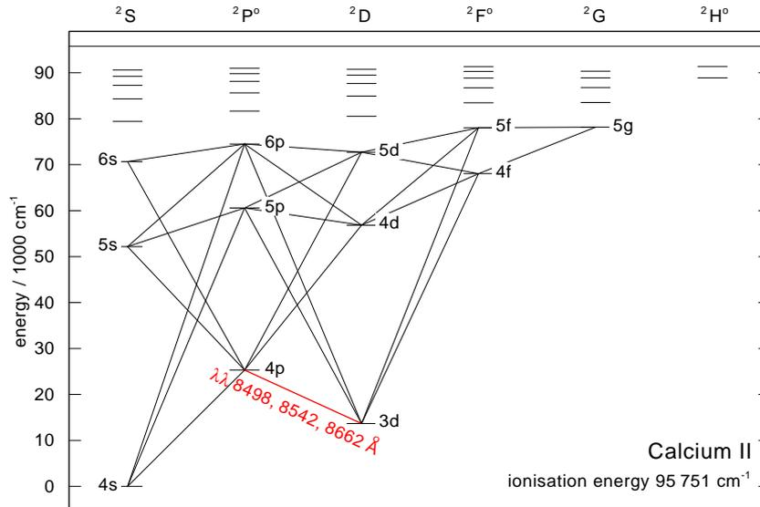
**Figure 1.** Grotrian diagram of our Ca II model ion. All highly excited levels that are not linked by radiative line transitions are treated in LTE. The 3d–4p transition causes the observed IR triplet.
