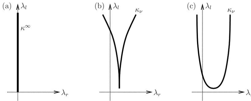
**Figure 6.** Solution curves of (63) and (62) in the  $(\lambda_r, \lambda_l)$ -plane for fixed  $\nu$ . Panel (a) shows the solution curve  $\kappa^\infty$  of the unperturbed equation (63), which is a simple parabola in the  $(\lambda_l, u)$ -plane and a ray in the  $(\lambda_r, \lambda_l)$ -plane that is covered twice as  $u$  is varied. Panels (b) and (c) show possible perturbations of  $\kappa^\infty$ .
