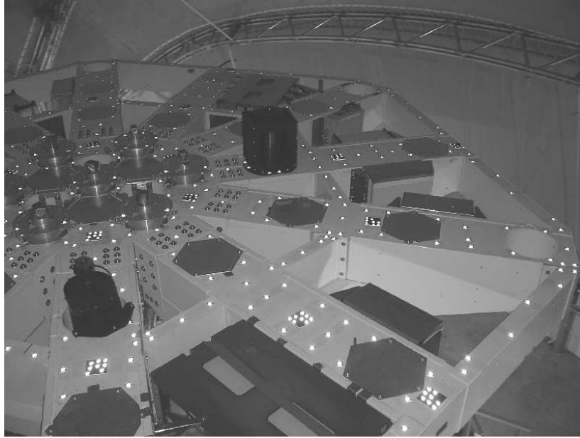
Figure 2. OT1 (in the back) and OT2 (in the front, lower left hand side corner), mounted with a 90^\circ phase shift in between them at a radius of 1.4m. Clearly seen are also the reflecting photogrammetry targets.
