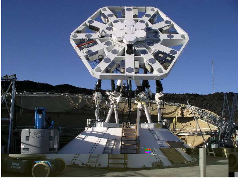
Figure 1. Front view of the AMiBA. Installed are 7 antennas in compact configuration, giving 0.6m, 1.04m and 1.2m baselines. Free receiver holes in the platform allow for different array configurations and for the expansion phase with 13 antennas. The 1st 8 inch refractor (OT1) for optical pointing is attached to the black bracket below the lowermost antenna at a distance of 1.4m from the platform center. A second optical telescope (OT2) is located at 90^\circ to the left hand side at the same radius.
