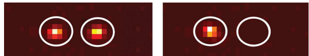
FIG. 4. Left : Fluorescence image of two \text{Ba}^+ ions. Right : Fluorescence of one ^{138}\text{Ba}^+ next to an unknown dark ion. We infer the existence of the dark ion from the position of the \text{Ba}^+ .
