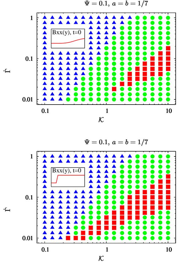
FIG. 16: Initial conditions dependency in the plane  $(\dot{\Gamma}, \mathcal{K})$ , using  $a = b = 1/7$  and  $\Psi = 0.1$ . In the upper graph we considered sigmoidal initial conditions, and in the lower graph step-like ones. In both cases, the amplitude of the strain inhomogeneities was reduced to 10% in amplitude, whereas Fig. 12 corresponded to 500% to enhance the effect.
