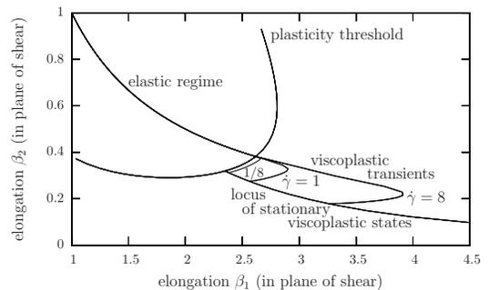
FIG. 10: Form of the stored elastic deformation in the course of an experiment and in the stationary regime, for three different values of the shear rate  $\dot{\gamma}$ . The axes are the first two eigenvalues,  $\beta_1$  and  $\beta_2$ , of tensor  $B$ .
