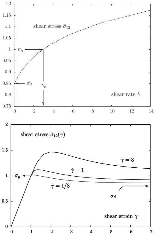
FIG. 9: Top: typical stationary flow curve. Points corresponding to  $\sigma_d$ ,  $\sigma_y$  and  $\dot{\gamma}_c$  are reported on the curve. Bottom: stress time evolution for different imposed shear rates below or above  $\dot{\gamma}_c$ .
