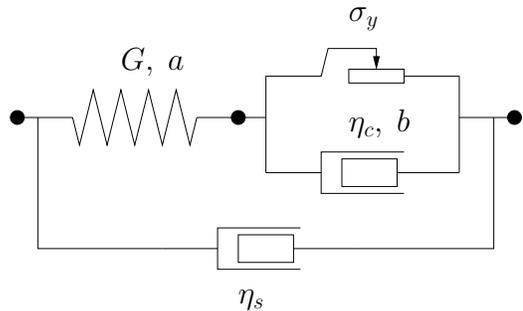
FIG. 4: Simplified (scalar) picture of the main rheological parameters.  $G$  represents the elastic modulus and  $a$  the relative weight of the tensorial components of the elastic deformation, see Eqs. (27) and (28). The quantities  $\sigma_y$  and  $1/\tau$  constitute a scalar representation of the creep defined by  $D_p^B$ , and parameter  $b$  is the equivalent of  $a$  for creep, see equation (31). Finally,  $\eta_s$  is a viscosity that is independent of creep.
