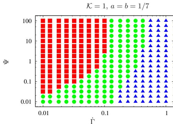
FIG. 13: Comparison of 0D and 1D simulations in plane  $(\dot{\Gamma}, \Psi)$ , using  $a = b = 1/7$  and  $\mathcal{K} = 1.0$ . Blue triangles indicate values for which the 0D model allows only uniform flow. Red squares indicate values for which shear banding was obtained in the 1D simulation for the initial conditions chosen. Green disks indicate additional values for which the 0D model allows shear banding.
