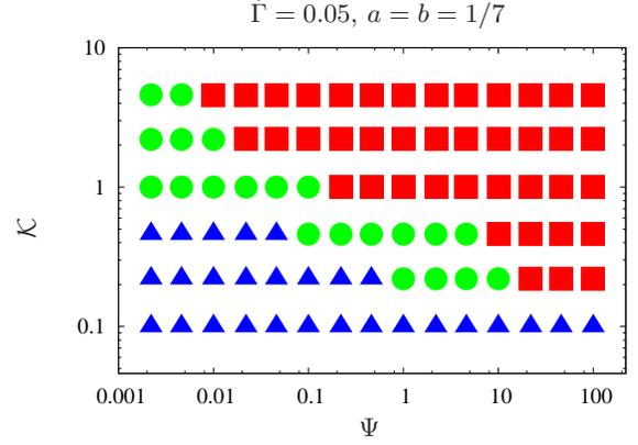
FIG. 11: Comparison of 0D and 1D simulations in plane  $(\mathcal{K}, \Psi)$ , using  $a = b = 1/7$  and  $\dot{\Gamma} = 0.05$ . Blue triangles indicate values for which the 0D model allows only uniform flow. Red squares indicate values for which shear banding was obtained in the 1D simulation for the initial conditions chosen. Green disks indicate additional values for which the 0D model allows shear banding.
