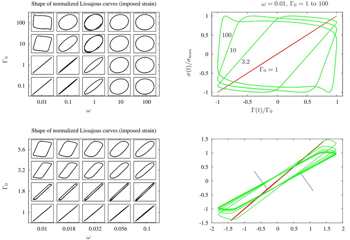
FIG. 5: Large amplitude oscillatory simulations: shape of  $\Gamma(t)$  versus  $\sigma_{xy}(t)$  (Lissajous) curves, obtained for  $a = b = 1/7$ ,  $\Psi = 0.1$  and  $\mathcal{K} = 1$ . Top: range from  $\omega = 0.01$  to  $\omega = 100$  and  $\Gamma_0 = 0.1$  to  $\Gamma_0 = 100$ . Bottom: zoom on a more restricted range of parameters.
