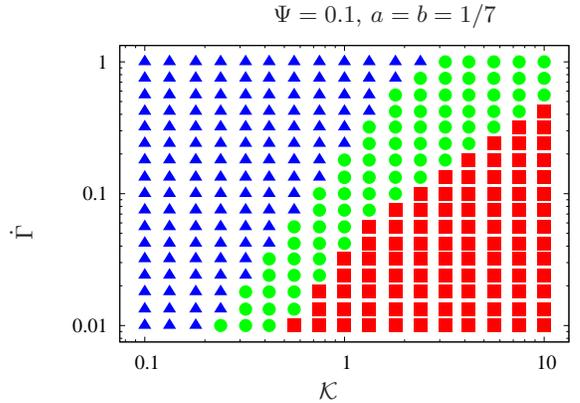
FIG. 12: Comparison of 0D and 1D simulations in plane  $(\dot{\Gamma}, \mathcal{K})$ , using  $a = b = 1/7$  and  $\Psi = 0.1$ . Blue triangles indicate values for which the 0D model allows only uniform flow. Red squares indicate values for which shear banding was obtained in the 1D simulation for the initial conditions chosen. Green disks indicate additional values for which the 0D model allows shear banding.
