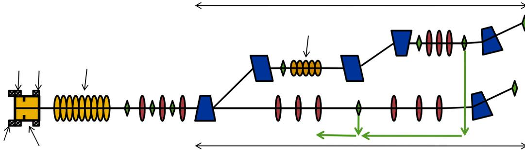
FIG. 1. Top view of the A0 Photoinjector showing elements pertinent to performing emittance exchange. Elements labeled “X” are diagnostics stations (beam viewers and/or multi-slit mask locations), “S” are solenoid lenses, “Q” are quadrupole magnets and “D” are dipole magnets.
