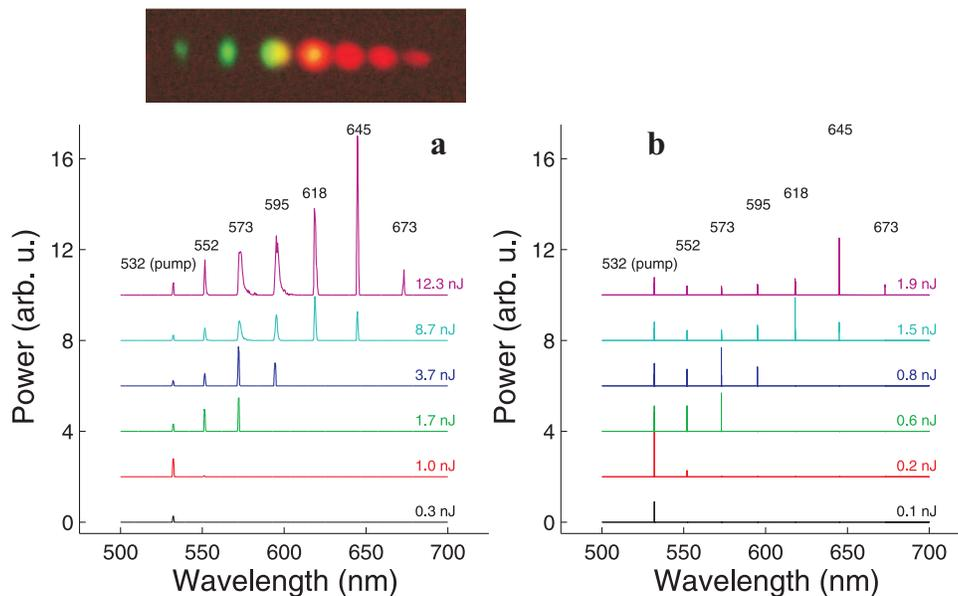
FIG. 2. (color online). Experimental and simulation results for 532nm pumping. Measured a) and calculated b) evolution of the output spectrum as the pump pulse energy is increased, for a pump wavelength of 532 nm. Inset of a): Photograph of the Raman lines separated in space using a prism.
