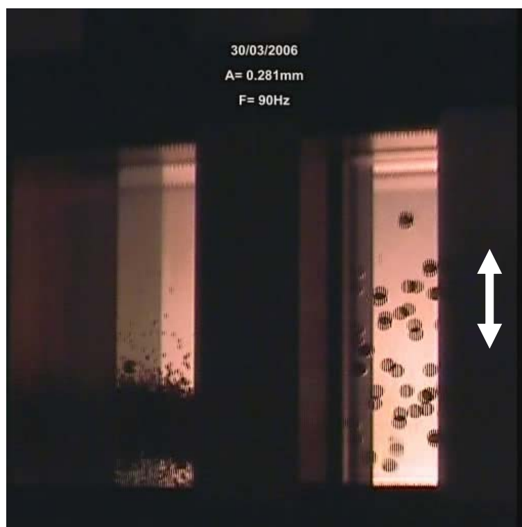
Figure 4: The Maxus rocket cell recorded via the camcorder during 0g period in Airbus A300-0g (30/3/2006), amplitude A=0.281\text{mm} , frequency f=90\text{Hz} ; the 2d cell is the right one. As the camcorder record each frame by recording 2 half of frames separated by the half duration existing between two frames, each photo appears as the sum on the two complementary half frames. So the balls appear twice separated by the distance it moves during half a frame; the position of the ball is then the average between these two positions. This Fig.4 is added from the original text of the Sino-German seminar.
