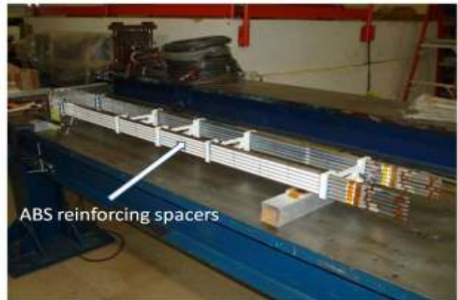
Fig. 9 Magnet power cable with ABS spacers strengthening cold pipes.
