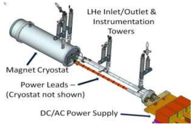
Fig. 8 Cryogenic system; leads cryostat is hidden to show lead structure.
