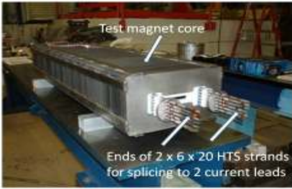
Fig. 11 Coil inside core and HTS strand ends to be spliced to current leads.
