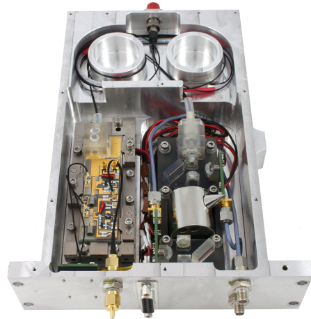
Fig. 5 The rubidium spectroscopy module for the FOKUS payload with open cover. The frequency of a DFB laser (left) is stabilized to the rubidium gas cell on the optical bench (right). Electronic interfaces for module operation are on the front and the fiber interface with the frequency comb is located on the rear side. The dimensions are 215 mm×170 mm×50 mm and the total mass is 2.1 kg.
