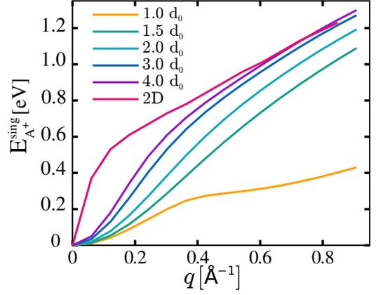
FIG. 5. Dispersion of the visible “A<sup>+</sup>” exciton for different interlayer distances  $d$  ( $d_0$  is the experimental value). For each case the exciton energies are defined with respect to the corresponding  $q = 0$  value.
