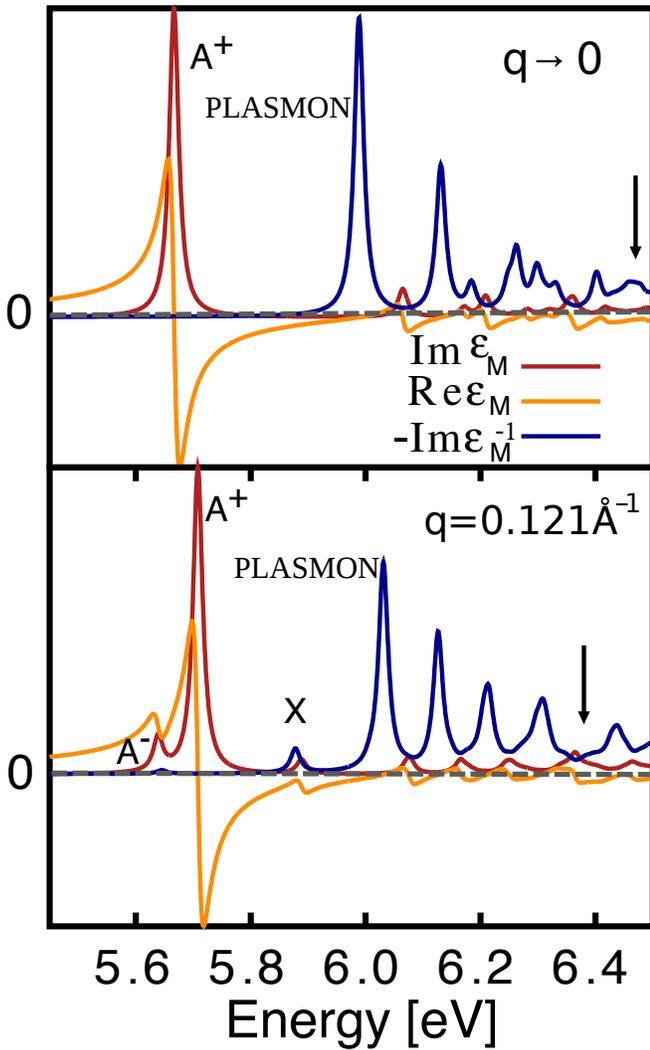
FIG. 1. The real and imaginary parts of the macroscopic dielectric function  $\text{Re}\epsilon_M$  and  $\text{Im}\epsilon_M$  and the loss function  $-\text{Im}\epsilon_M^{-1}$  calculated at two different wave vectors  $\mathbf{q}$  along the in-plane  $\Gamma M$  direction. For improved visibility the loss functions have been rescaled. The vertical arrows mark the smallest independent-particle GW transition energy (which for  $\mathbf{q} = 0$  corresponds to the direct band gap).
