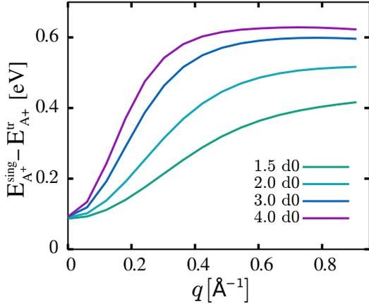
FIG. 7. Energy difference between the singlet and triplet “A<sup>+</sup>” excitons as a function of momentum  $\mathbf{q}$  for different interlayer distances.
