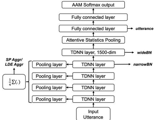
Figure 2: The x-vector model and the various types of embedding that are extracted from its layers. The TDNN and fully connected layers, if not marked, are all 512-dimensional. ‘AAM softmax’ denotes *additive angular margin softmax* [47]. The pooling layer on the left-hand side can be either statistics pooling or learnable dictionary encoding (LDE).
