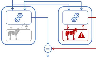
Fig. 2. Two instances of the same IP (“miter”), both containing an HT. The same inputs are fed to both instances. The HT in instance<sub>1</sub> is triggered while the HT in instance<sub>2</sub> is dormant. This results in an observable difference in the behavior of the two IPs.
