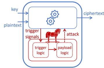
Fig. 1. HT in a cryptographic IP. The HT consists of a trigger and payload.
