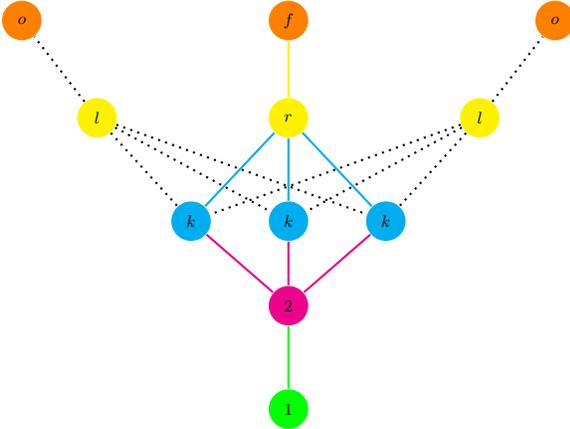
Figure 1. *Lily Graph* topology – The *input nodes* ( $|1\rangle$  and  $|2\rangle$ ) are green and magenta labeled, the *chiral layer* ( $|k\rangle$ ), composed of  $d$  nodes, is blue labeled, the *routing layer* ( $|l\rangle$  and  $|r\rangle$ ) composed of  $n$  vertices (yellow labeled) and accordingly the  $n$  outputs ( $|f\rangle$  and  $|o\rangle$ ) are orange labeled.
