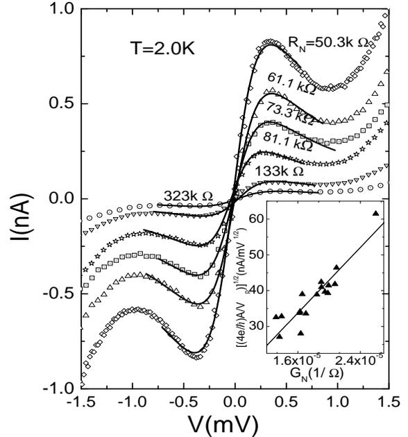
FIG. 3. Low bias current-voltage characteristics for various junction resistances at  $T = 2.0 \text{ K}$ . The data (points skipped for clarity) is represented by symbols, and the lines represent two-parameter fits to theory. Inset-  $I_{c,0} \times \sqrt{e/k_B T}$  vs.  $G_N$  (see text).
