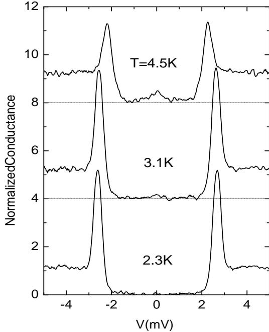
FIG. 2. Normalized  $dI/dV$  curves for a high resistance ( $R_N = 100 \text{ M}\Omega$ ) S/I/S junction at various temperatures. Curves offset for clarity, horizontal lines correspond to zero conductance of each curve.
