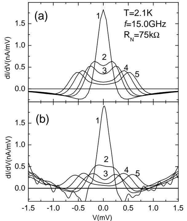
FIG. 4. (a) Calculation of the conductance at low bias voltages due to Josephson tunneling in the presence of microwave fields ( $f = 15.0$  GHz) for various induced ac voltages on the junction. (b) Numerically differentiated current-voltage data for a junction with  $R_N = 75$  k $\Omega$  at  $T = 2.1$  K. Curves 1-5 correspond to  $V_{ac} = 0, 0.31, 0.39, 0.54,$  and  $0.65$  mV respectively.
