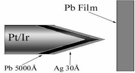
FIG. 1. Schematic depiction of the experimental setup.
