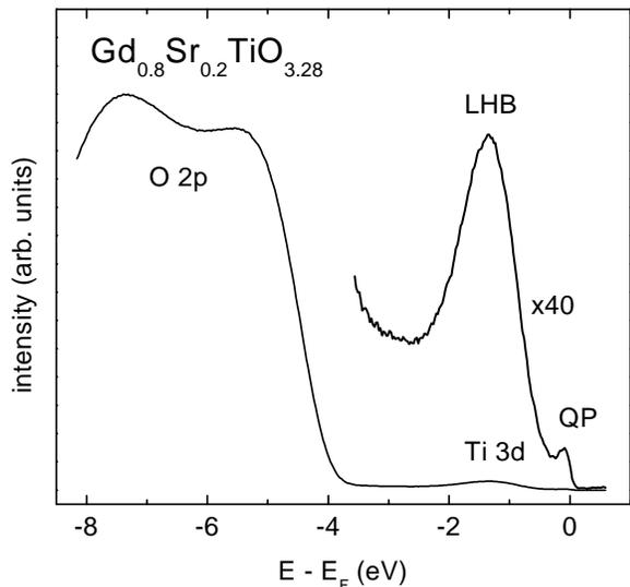
FIG. 1: UPS valence band spectrum of  $\text{Gd}_{0.8}\text{Sr}_{0.2}\text{TiO}_{3.28}$ . The spectrum has been corrected for He  $I_{\beta}$  satellite emission. The Ti 3d-derived part of the spectrum decomposes into the lower Hubbard band (LHB) and a quasiparticle peak (QP) at the Fermi level.
