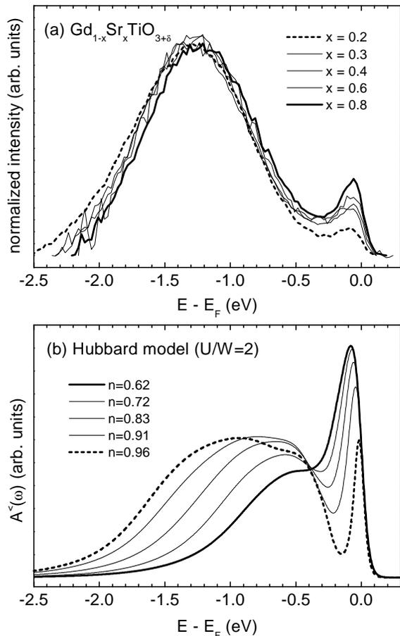
FIG. 2: (a) Ti 3d spectra of  $\text{Gd}_{1-x}\text{Sr}_x\text{TiO}_{3+\delta}$  with varying Sr-doping. For better clarity an inelastic background is subtracted. The spectra are normalized to same integral Ti 3d weight. (b) Theoretical photoemission spectra  $A^{<}(\omega)$  calculated for the Hubbard model at various band filling factors  $n$ . The ratio of on-site Coulomb energy  $U$  and band width  $W$  is chosen as  $U/W = 2$ , with  $W$  set to 2 eV. See text for further details.
