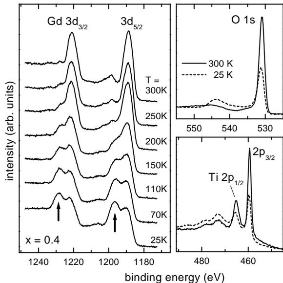
FIG. 3: XPS core level spectra of  $\text{Gd}_{0.6}\text{Sr}_{0.4}\text{TiO}_{3.28}$ . Left panel: Temperature-dependence of the Gd  $3d$  spectra. Note the evolution of an additional structure (denoted by arrows) below 200 K. Right panels: O  $1s$  and Ti  $2p$  spectra of the same sample at room temperature (solid line) and 25 K (dashed line).
