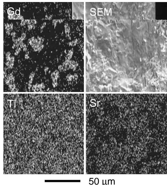
FIG. 4: Scanning electron micrograph of a scraped surface of polycrystalline  $\text{Gd}_{0.7}\text{Sr}_{0.3}\text{TiO}_{3.3}$ , measured with a primary electron energy of 20 keV (upper right panel). Also shown are the elemental maps for Gd, Ti, and Sr simultaneously obtained by EDX. White (black) areas denote high (low) concentration.
