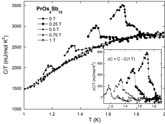
FIG. 2: Specific heat divided by temperature  $C/T$  versus  $T$  between 1 and 2 K in magnetic fields up to 1 T for an individual single crystal sample of  $\text{PrOs}_4\text{Sb}_{12}$ . The data for fields below 1 T have been truncated below the superconducting transitions for clarity. Inset:  $\Delta C/T$  versus  $T$ , where  $\Delta C = C(H, T) - C(H = 1\text{T}, T)$ .
