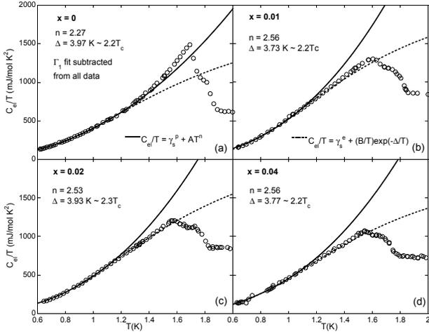
FIG. 6: Comparison of exponential (dashed line) and power law (solid line) fits below  $T_c$ , after subtracting lattice and Schottky anomaly terms for a  $\Gamma_1$  ground state, for  $\text{Pr}(\text{Os}_{1-x}\text{Ru}_x)_4\text{Sb}_{12}$  with (a)  $x = 0$ , (b)  $x = 0.01$ , (c)  $x = 0.02$ , and (d)  $x = 0.04$ . The  $x = 0$  fits only extend up to  $\sim 1.2$  K, while the  $x = 0.01$ ,  $x = 0.02$ , and  $x = 0.04$  fits only extend up to  $\sim 1.15$  K, as described in the text.
