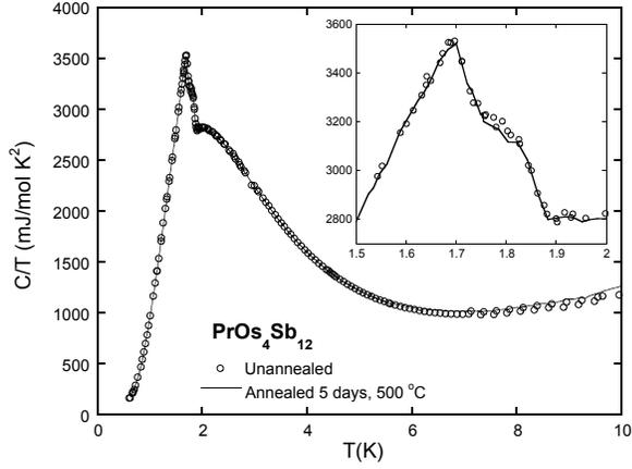
FIG. 1: Specific heat divided by temperature  $C/T$  versus  $T$  below 10 K for an unannealed set of single crystals of  $\text{PrOs}_4\text{Sb}_{12}$  (open circles) and the same sample annealed for 5 days at  $500^\circ\text{C}$  (solid line). Inset: close-up of the double superconducting transition. There is almost no difference between the two data sets.
