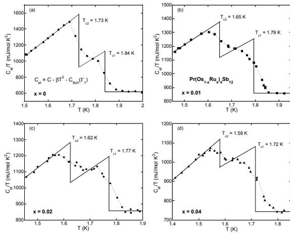
FIG. 4: Comparison of double superconducting transitions in  $C_{el}/T$ , after lattice and Schottky anomaly terms corresponding to a  $\Gamma_1$  ground state have been subtracted, for  $\text{Pr}(\text{Os}_{1-x}\text{Ru}_x)_4\text{Sb}_{12}$  with (a)  $x = 0$ , (b)  $x = 0.01$ , (c)  $x = 0.02$ , and (d)  $x = 0.04$ . The transitions were approximated with an entropy conserving construction.
