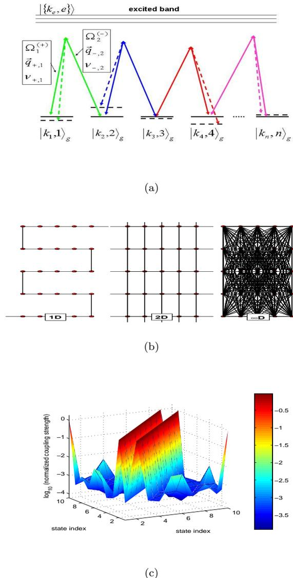
FIG. 1: (a) Proposed setup: the internal states of a cold atom (or molecule) are mixed by pairs of Raman beams and become entangled with different momentum states. Full lines indicate an ordered lattice of energies, dashed lines - a disordered lattice. (b) Momentum-space dimensionalities 1D, 2D,  $\infty D$ , illustrated by lattice graphs with different connectivities. (c) Numerical Raman coupling strengths in log scale for Li atoms in a 1D setup (for parameters at paper end).
